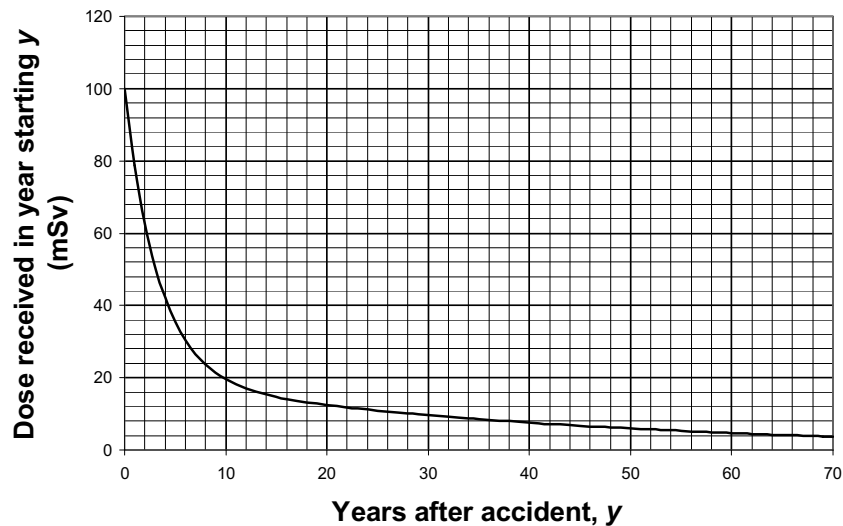
Fig. 5 – Dose profile for an external dose of 100 mSv in the year beginning 26 April 1986.
