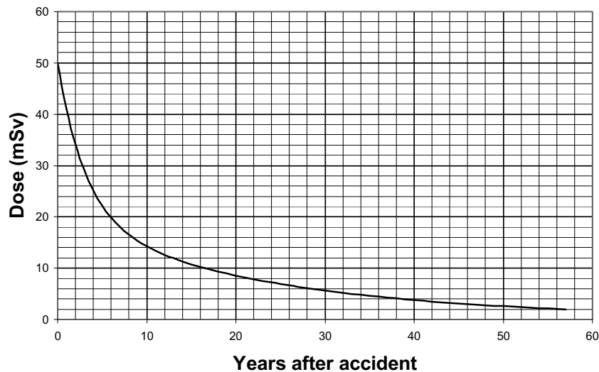
Fig. 10 – Dose received by people in a neighbouring town in the years after an imagined big nuclear reactor accident.
